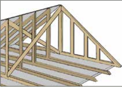
Figure 4-4. Diagonal braces form an X pattern from the top center of the gable end to the bottom center of the fourth truss and from the bottom center of the gable end to the top center of the fourth truss. The same screws as for lateral bracing are used. Source: FEMA's Against the Wind brochure 247.
