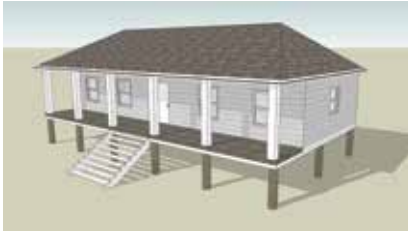
Figure 2-11. In this example, adding a small amount of height has very little effect on the look of a home, but results in a substantial flood insurance savings. 23 Image courtesy of MassCZM, more information available at www.mass.gov/czm/stormsmart/regulations/freeboard.htm
